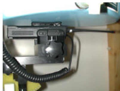
Figure 16. BODY SAR Test Setup w/ Belt Clip
