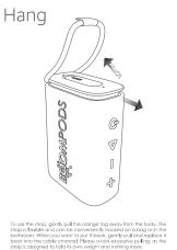
To use the strap, gently pull the orange tag away from the body. The strap is flexible and can be conveniently hocked on a bag or in the obthistorm. When you want to put it back, gently pull and replace it back into the cable channel. Please ovid excessive polling, as the strap is designed to hald its own weight and nothing more.
