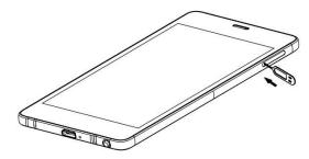
2. Insert the Micro-SIM card correctly in Micro-SIM Tray.
