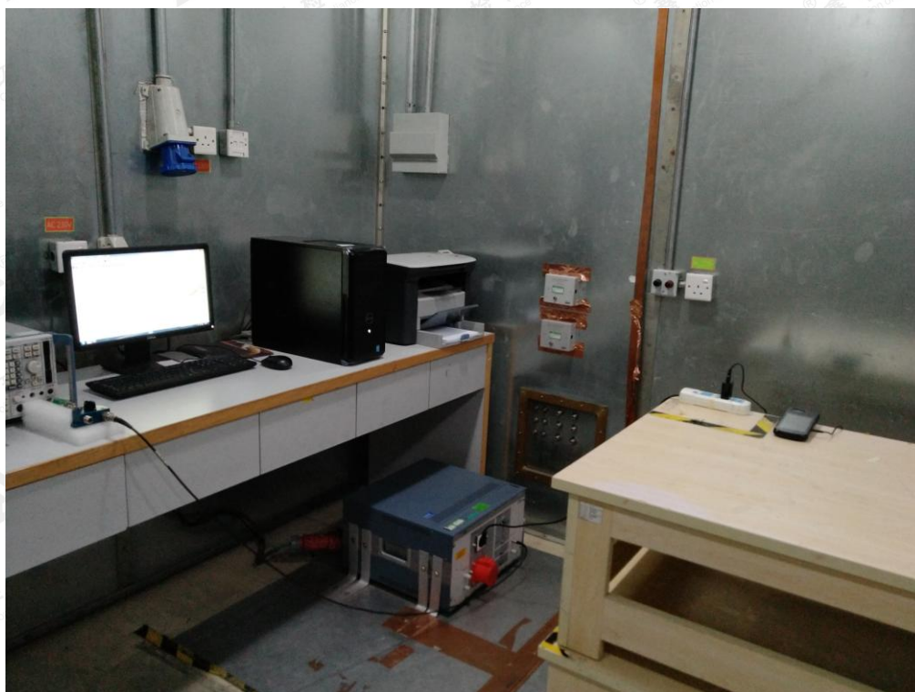
RADIATED EMISSION TEST SETUP
