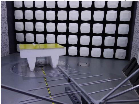
1.2 Radiated Emissions (Above 1GHz) Test Setup
