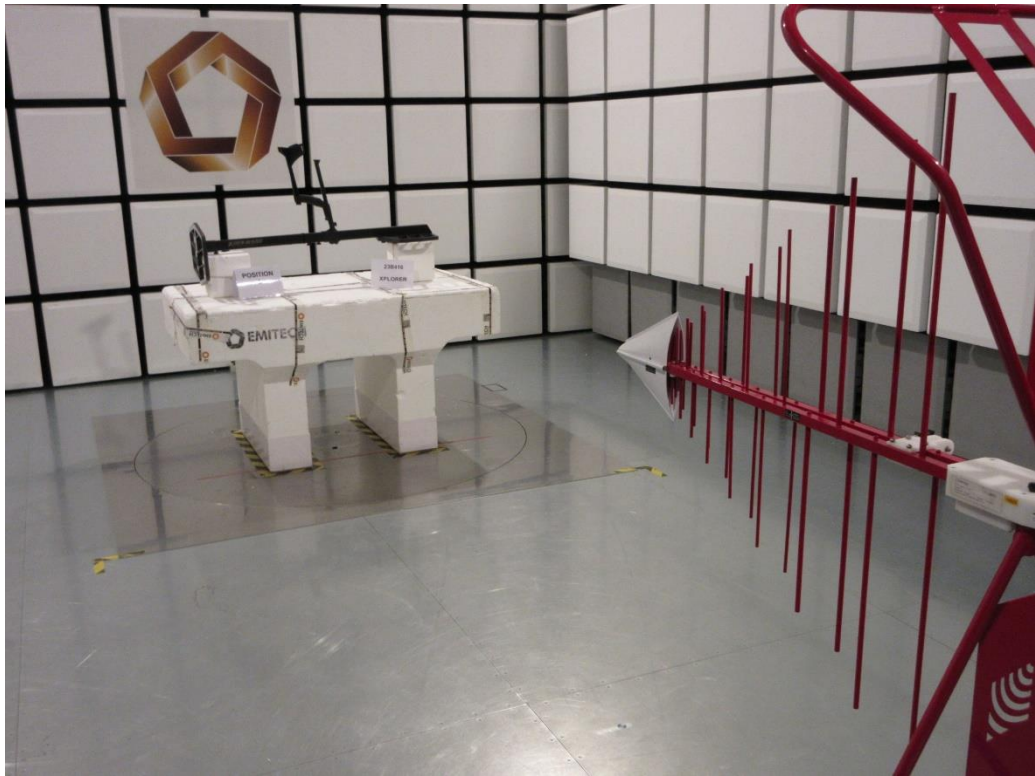
TEST SETUP PHOTO(S) – 30MHZ TO 1GHZ
