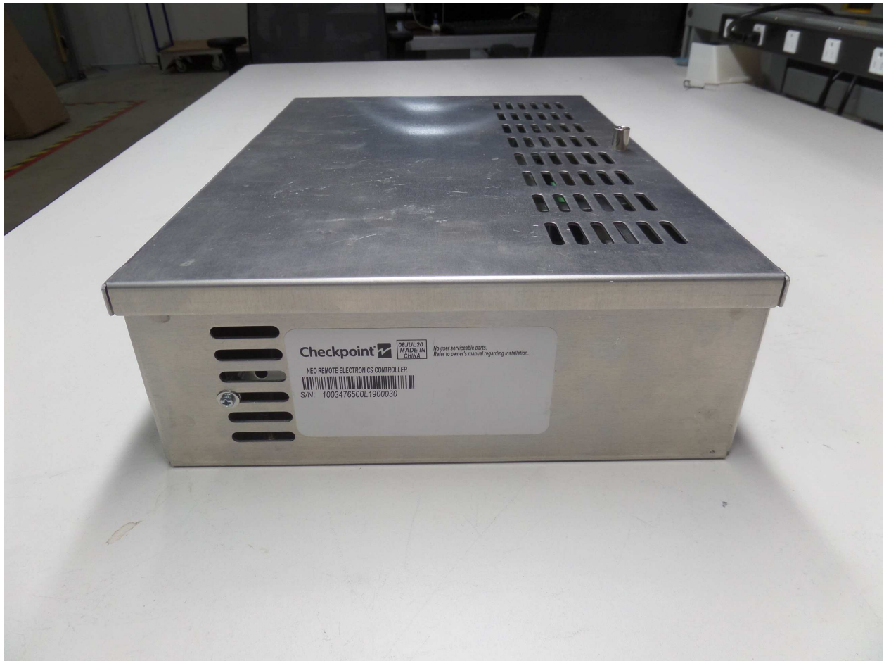
Label Location NEO Remote Electronics Controller
