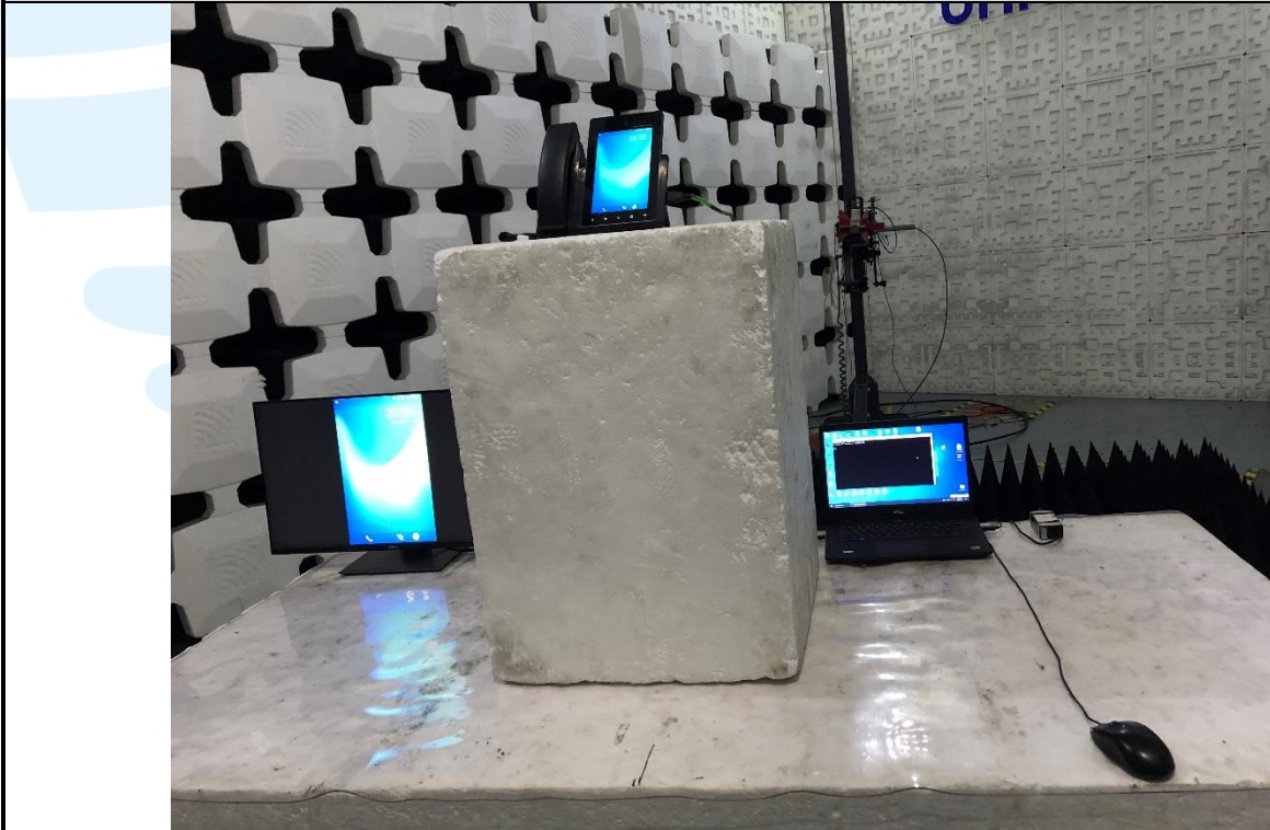
Radiated emission Test Setup (Above 1 GHz)
