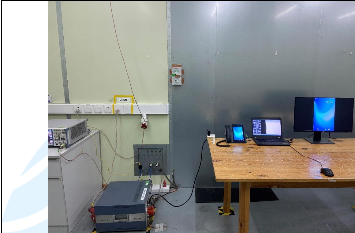
Conducted Emission Test Setup
