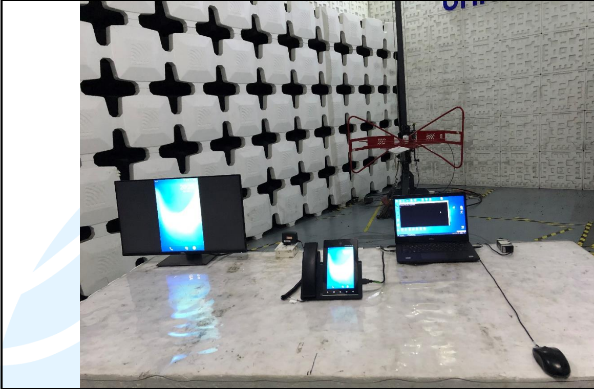
Radiated emission Test Setup (30 MHz~1 GHz)
