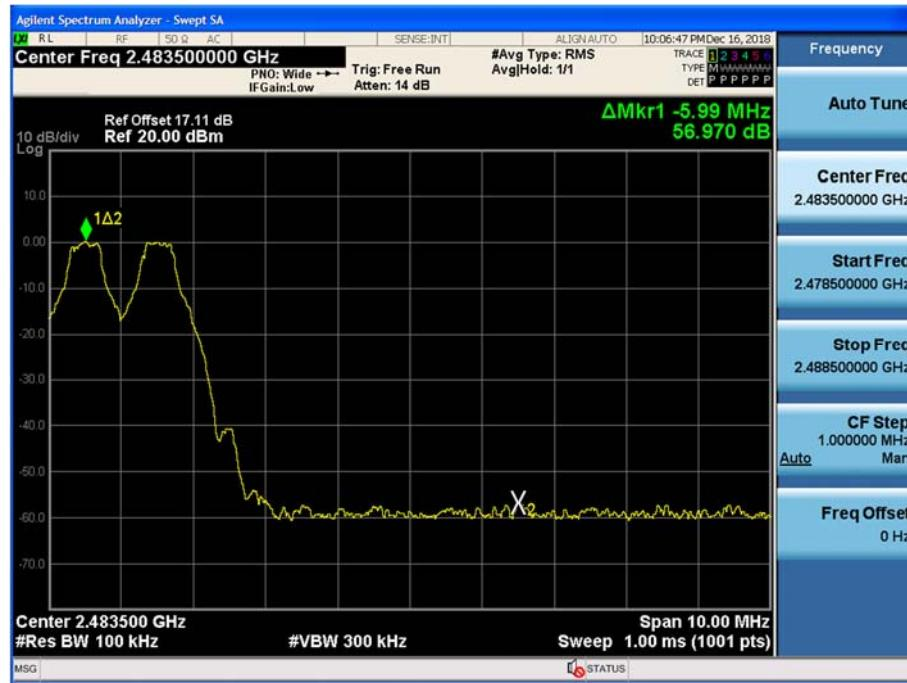
Test Plots with hopping (8DPSK)
