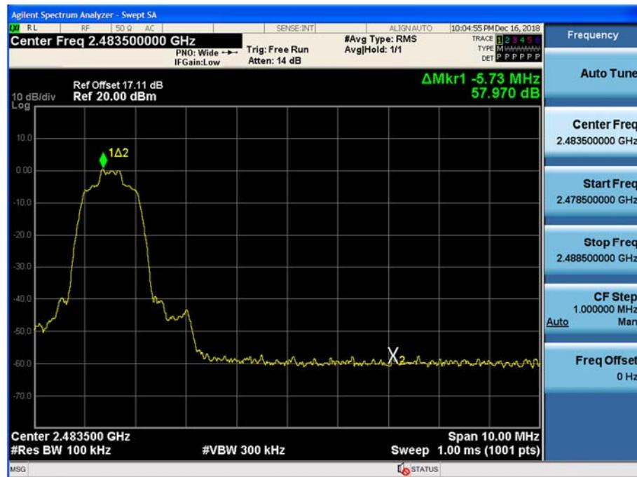
Test Plots with hopping (GFSK)
