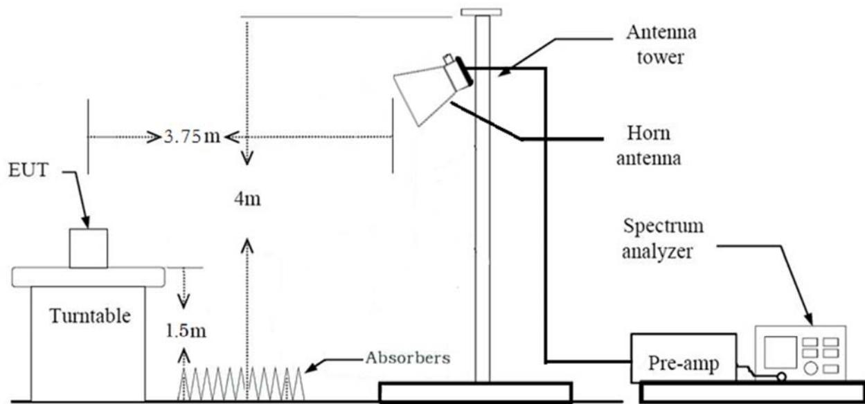
**Test Procedure of Radiated spurious emissions(Below 30 MHz)**
