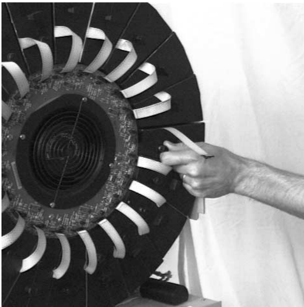
Figure 22-18. Disconnect the ribbon cable from the printed circuit board (donut)
