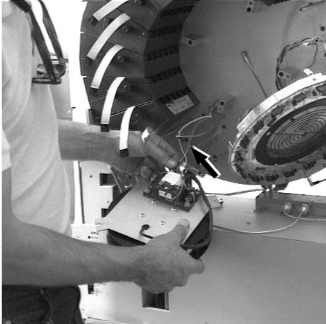
Figure 22-25. Remove and save silver standoffs and washers
