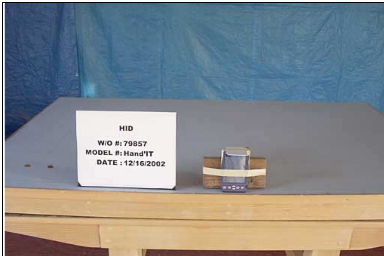
Radiated Emissions - Front View
