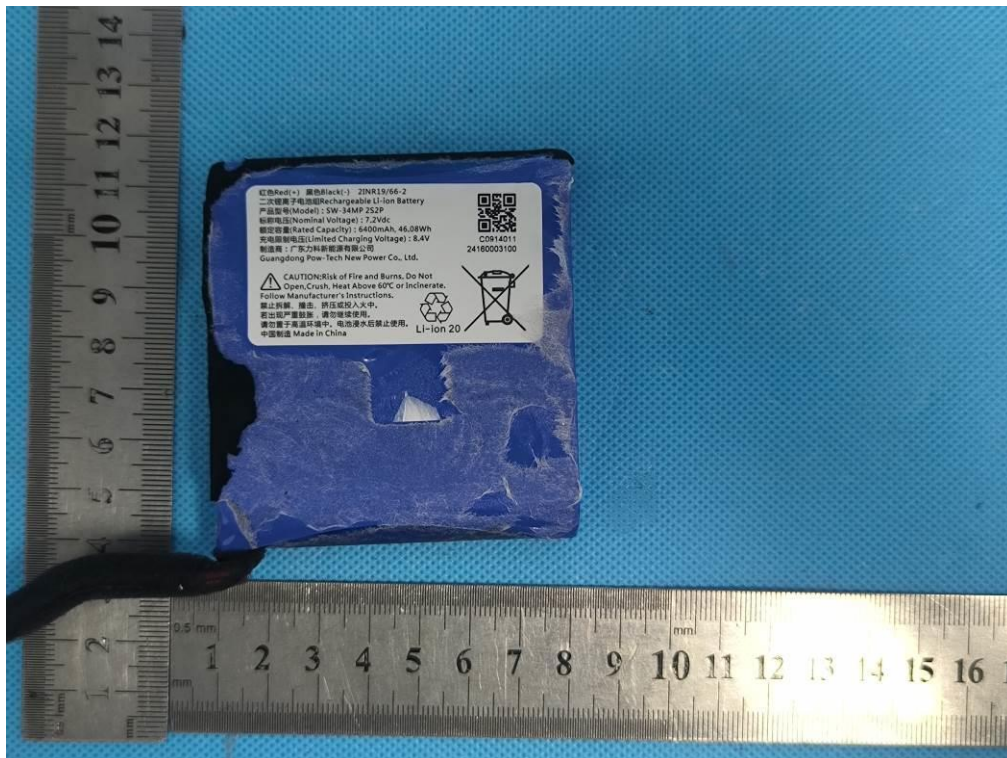
BATTERY VIEW OF EUT (FIGURE 1)
