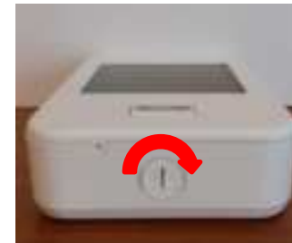
5 Place the battery tray cover and lock it by turning the lock key clockwise
