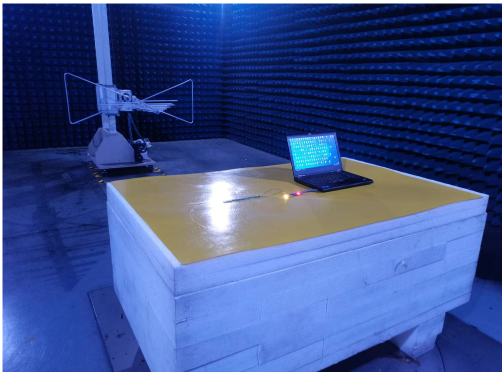
Photo of Radiated Emission Measurement (Above 1G)
