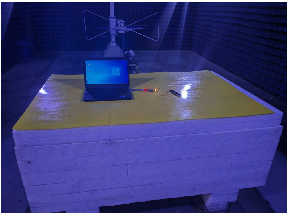
Photo of Radiated Emission Measurement (Above 1G)
