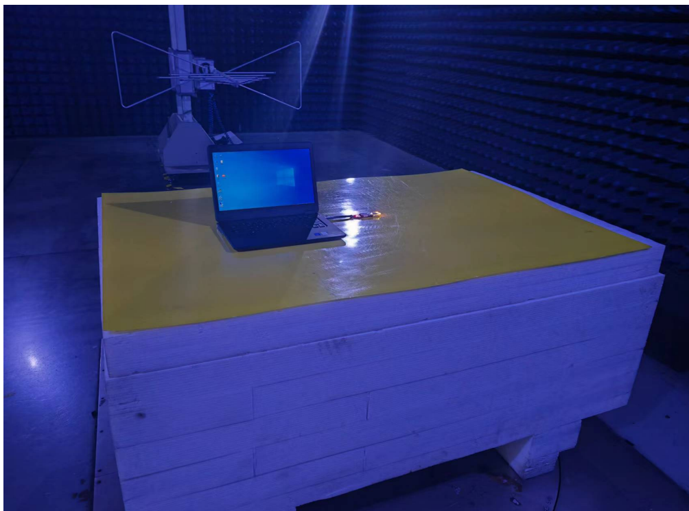
Photo of Radiated Emission Measurement (Above 1G)
