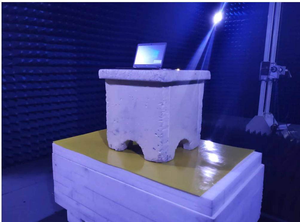
Photo of Radiated Emission Measurement (Above 1G)
