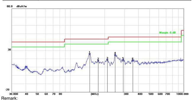
Factor = Antenna Factor + Cable Loss - Amplifier.
