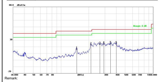
Factor = Antenna Factor + Cable Loss - Amplifier.
