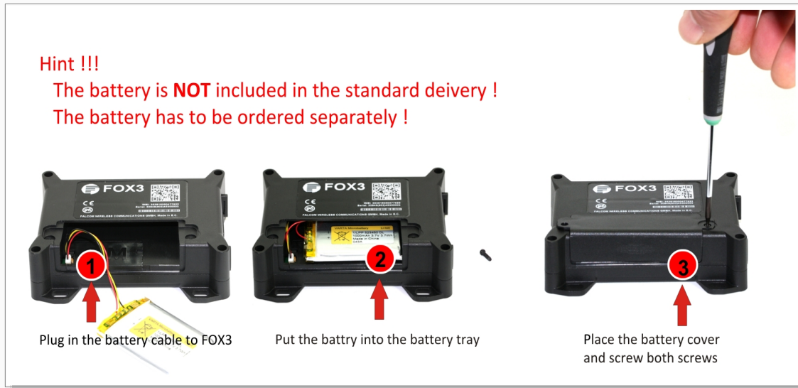
Figure 14.1: Connecting the battery to the FOX3-2G/3G/4G devices
