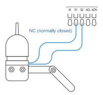
Insert the normally closed and common wires into the S1 and S2 terminal slots.
