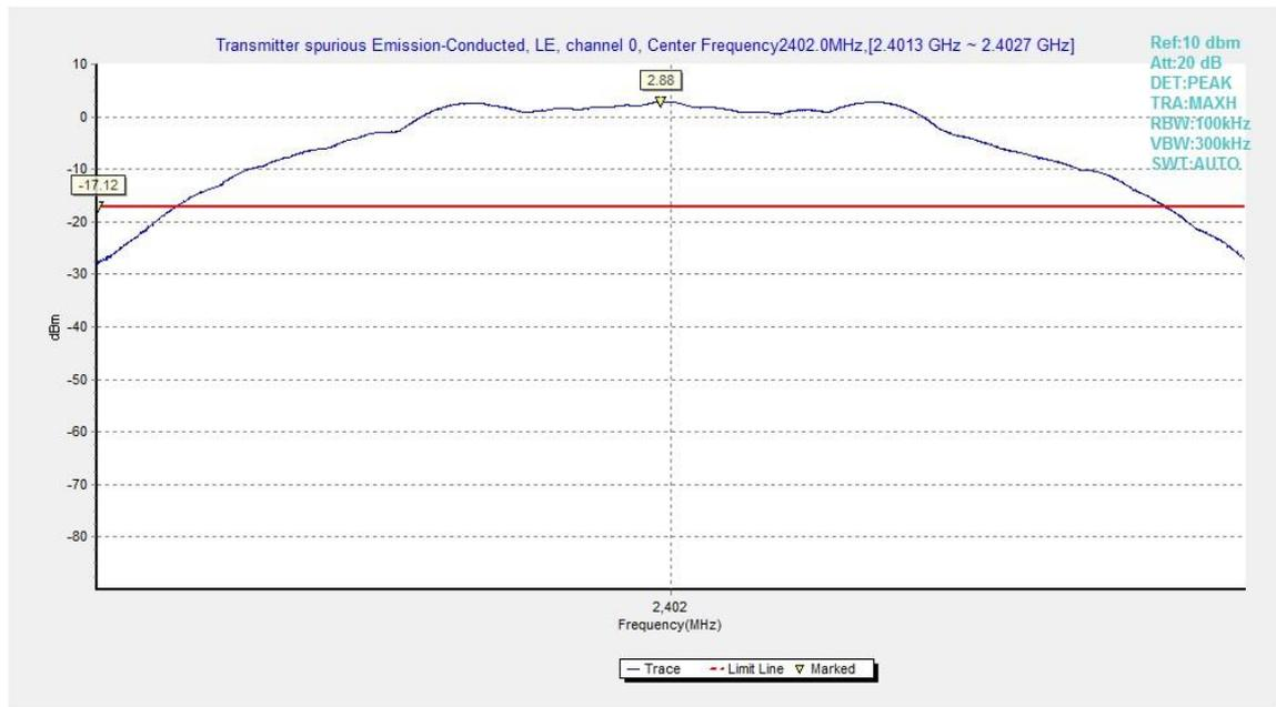
Fig.3. Transmitter Spurious Emission - Conducted: GFSK, 2402MHz
