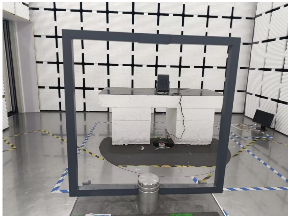
Radiation Emission Test Setup (Below 30MHz)
