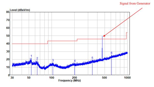
Site : chamber Condition: 3m VERTICAL Job No. : XMTN1220727-34211E-EM Test Mode: receiver at 462.6375MHz
