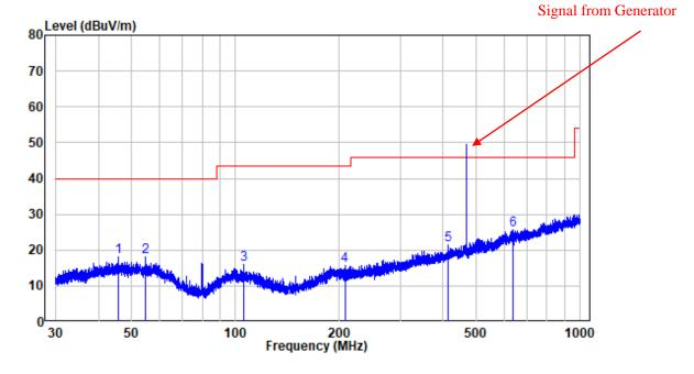
Site : chamber Condition: 3m HORIZONTAL Job No. : XMTN1220727-34211E-EM Test Mode: receiver at 467.6375MHz
