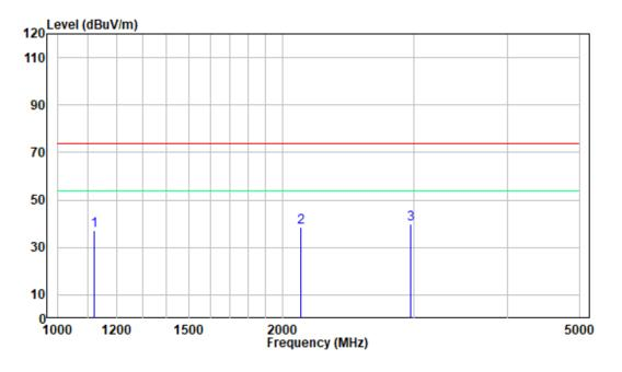
Site : chamber Condition: 3m VERTICAL Job No. : XMTN1220727-34211E-EM Test Mode: receiver at 462.6375MHz
