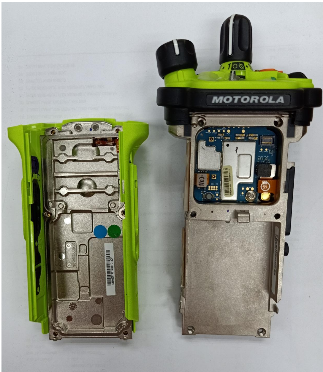
Expansion board with chassis and housing of APX6000XE Model 1.5 (Back side)
