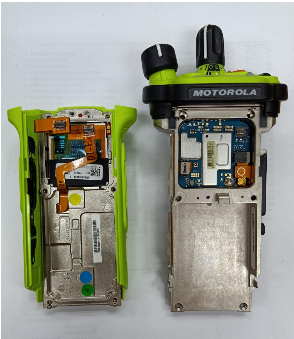
Expansion board with chassis and housing of APX6000XE Model 3.5 (Back side)
