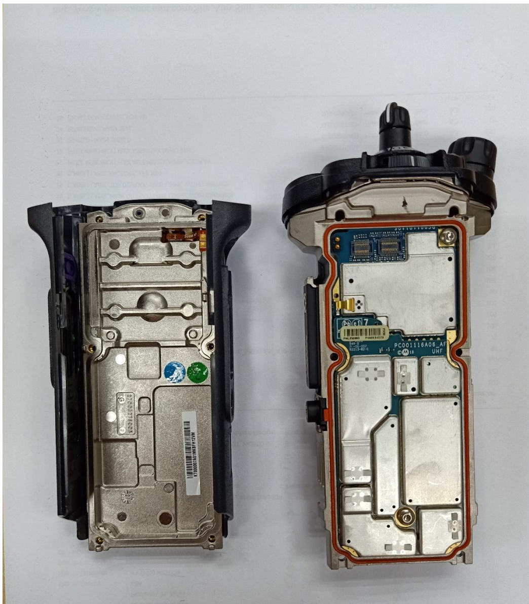
Expansion board with chassis and housing of APX6000/APX6000Li/APX5000 Model 1.5 (Back side)
