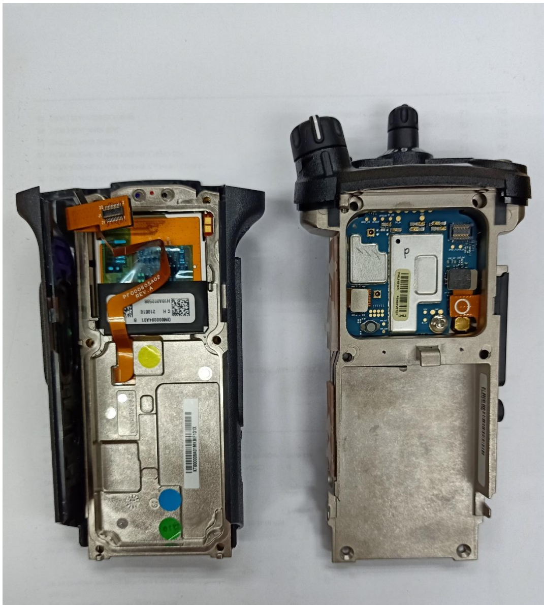
Expansion board with chassis and housing of APX6000/APX6000Li/APX5000 Model 3.5 (Back side)
