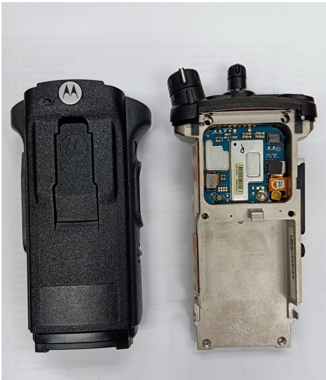
RF and Vocon boards with chassis and housing of APX6000/APX6000Li/APX5000 Model 1.5 (Front side)
