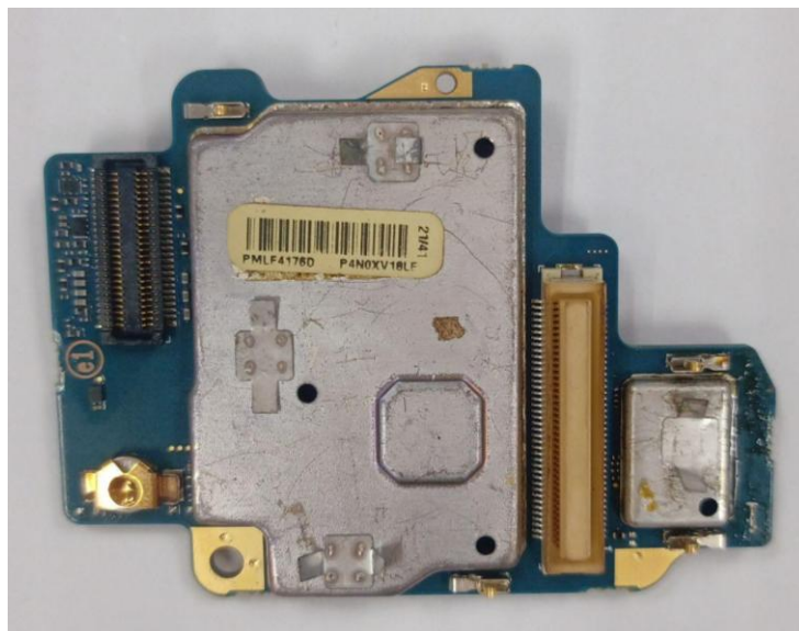
Vocon board with shields (Bottom) (APX6000/APX5000/APX6000XE/APX6000Li/SRX2200)
