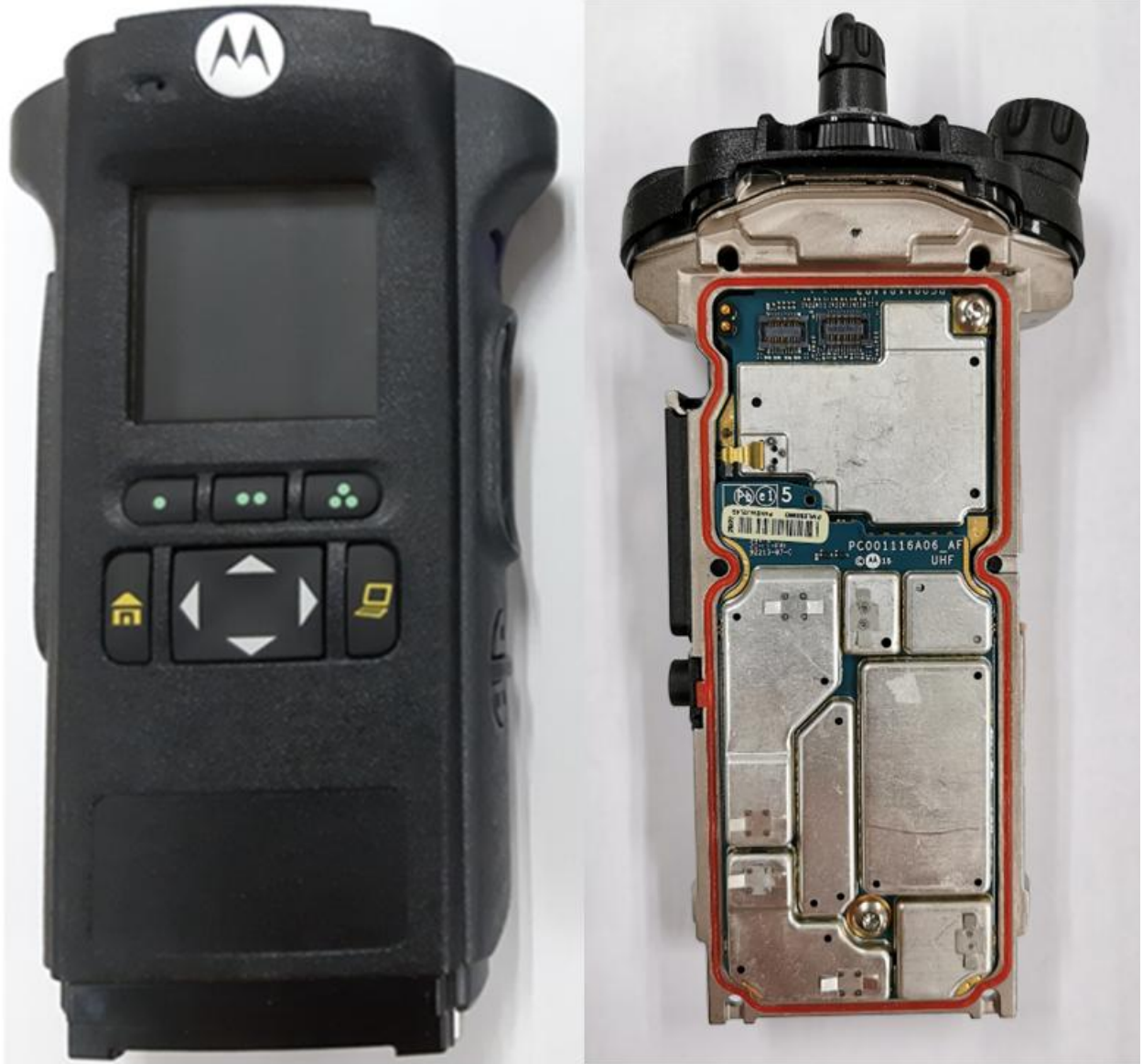
RF and Vocon boards with chassis and housing of APX6000/APX6000Li/APX5000 Model 2.5 (Front side)
