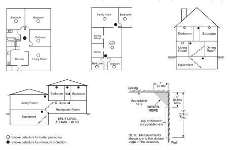
Smoke detectors should always be installed in accordance with NFPA 72, the National Fire Alarm Code. Smoke detectors should always be located accordance with the following:
