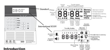
The RF5501-433 keypad combines a standard PC5132 receiver with an LCD5501Z keypad that presents system status using an LCD-style display with fixed messages. With the addition of the receiver portion, the control panel will now support up to 32 zones. The RF5501-433 is compatible with the following DSC security systems:
