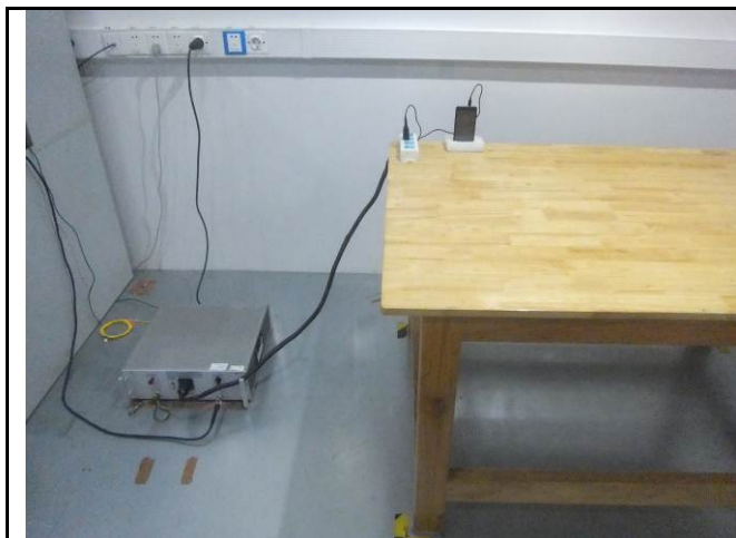
Conducted Emissions Test Setup Front View
