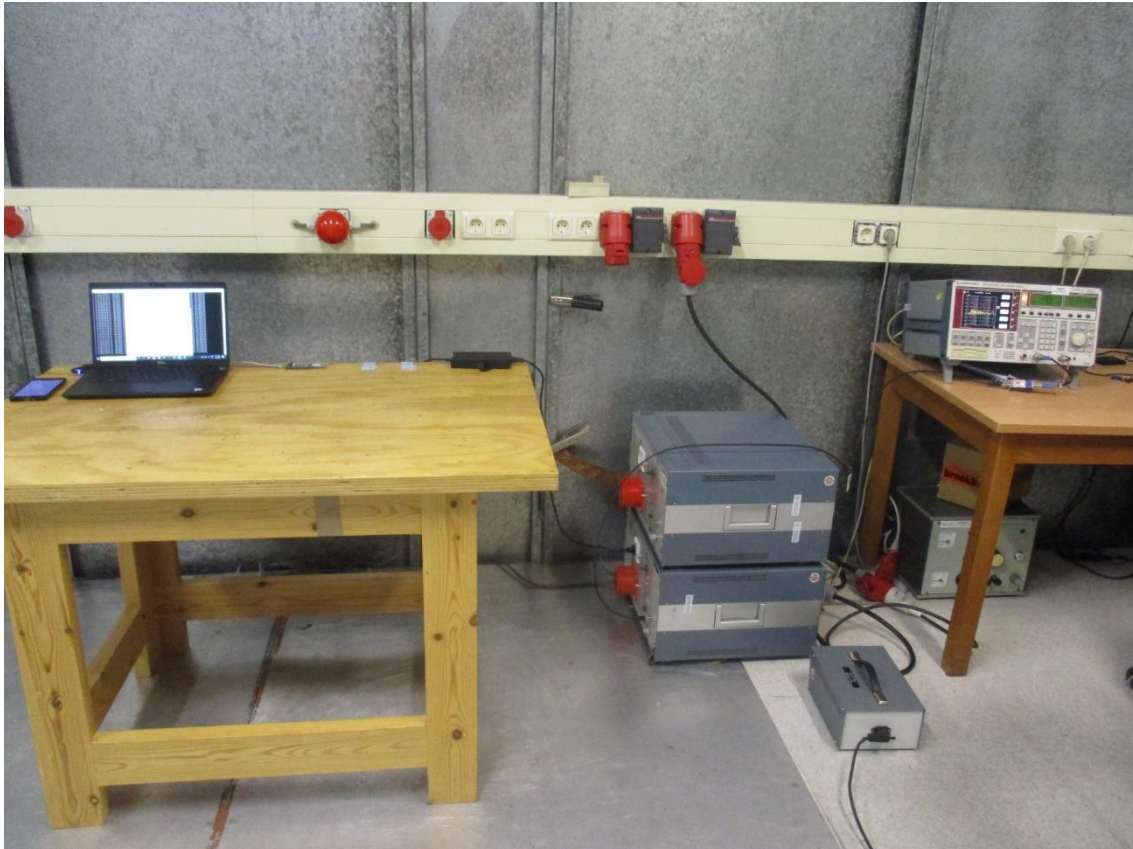
Photo 5: Photograph conducted emissions 0.15-30 MHz
