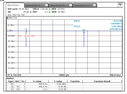
Note<sub>1)</sub> : period : 1 000.00 ms, On time : 996.60 ms Note<sub>2)</sub> : DCCF = 10 log(1 / x) = 10 log(996.60 / 1 000.00) = 0.01, x = 0.997 Note<sub>3)</sub> : 802.11a is a continuous transmission (duty cycle >=98 %)"
