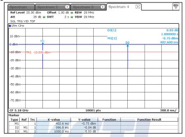
Note<sub>1)</sub>: period : 1 000.00 ms, On time : 996.80 ms Note<sub>2)</sub> : DCCF = 10  $\log(1 / x) = 10 \log(996.80 / 1 000.00) = 0.01$ , x = 0.997Note<sub>3)</sub> : 802.11a is a continuous transmission (duty cycle >=98 %)"
