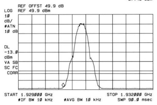
BLOCK EDGE (BLOCK A) (GSM MODULATION)
