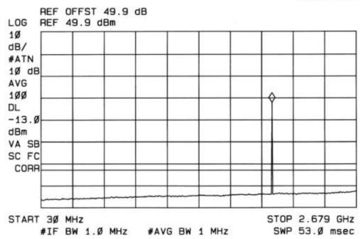
OUT OF BAND #1 1964.6MHz (EDGE MODULATION)
