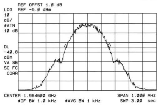
BANDWIDTH IN 1964.6MHz (GSM MODULATION)
