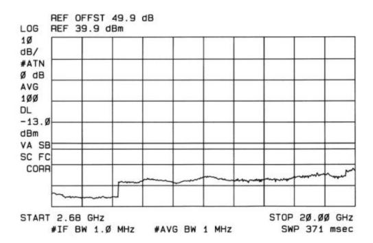
OUT OF BAND #2 1930.4MHz (EDGE MODULATION)
