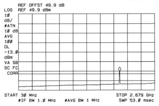
OUT OF BAND #1 1989.6MHz (GSM MODULATION)
