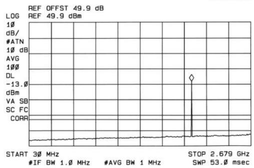
OUT OF BAND #1 1964.6MHz (GSM MODULATION)
