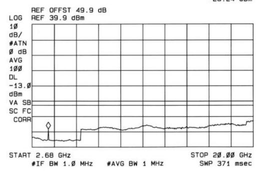
OUT OF BAND #2 1989.6MHz (EDGE MODULATION)
