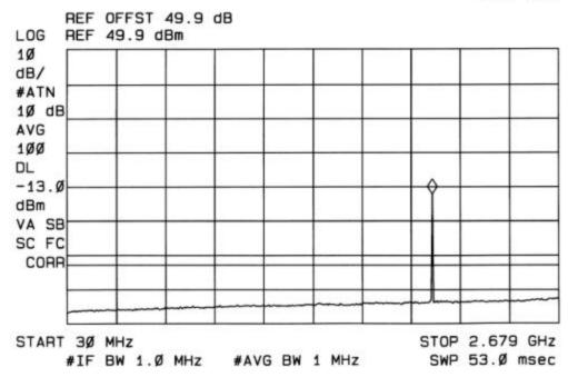
OUT OF BAND #1 1989.6MHz (EDGE MODULATION)
