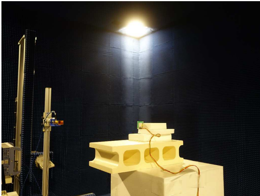
Photograph 8: Set-up for Radiated Spurious Emission above 40GHz, Rear View
