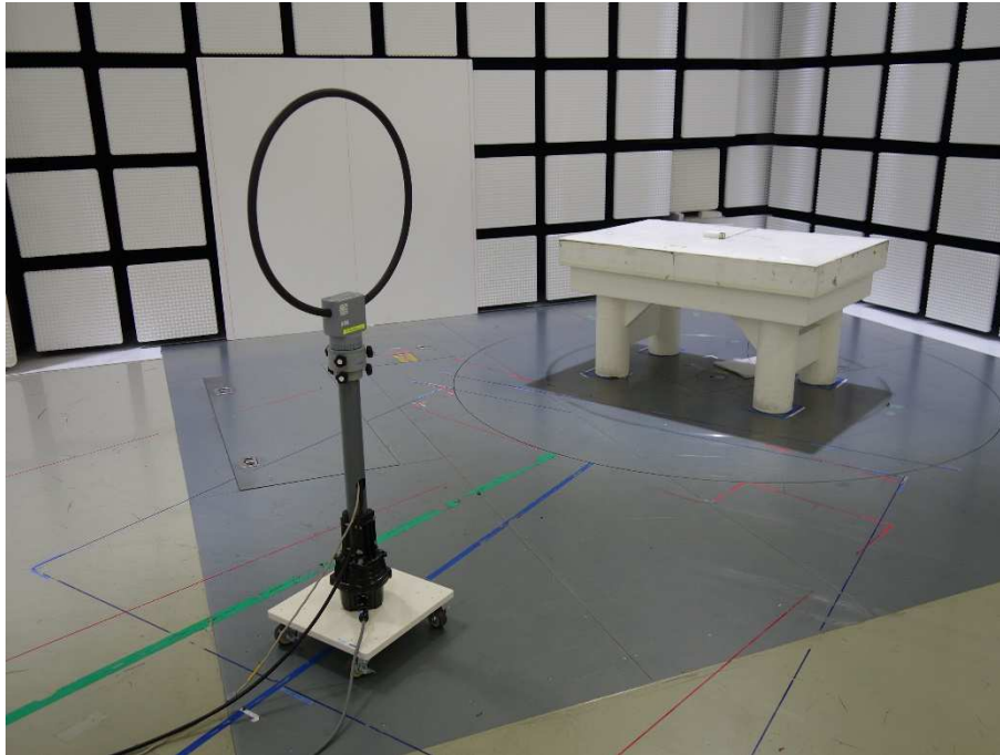
Photograph 1: Set-up for Radiated Spurious Emission below 30MHz, Front View
