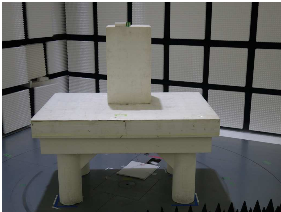
Photograph 5: Set-up for Radiated Spurious Emission above 1GHz, Front View
