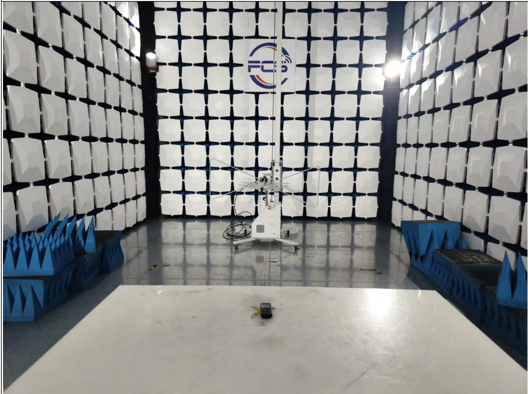
Above 1GHz for radiated emission test setup
