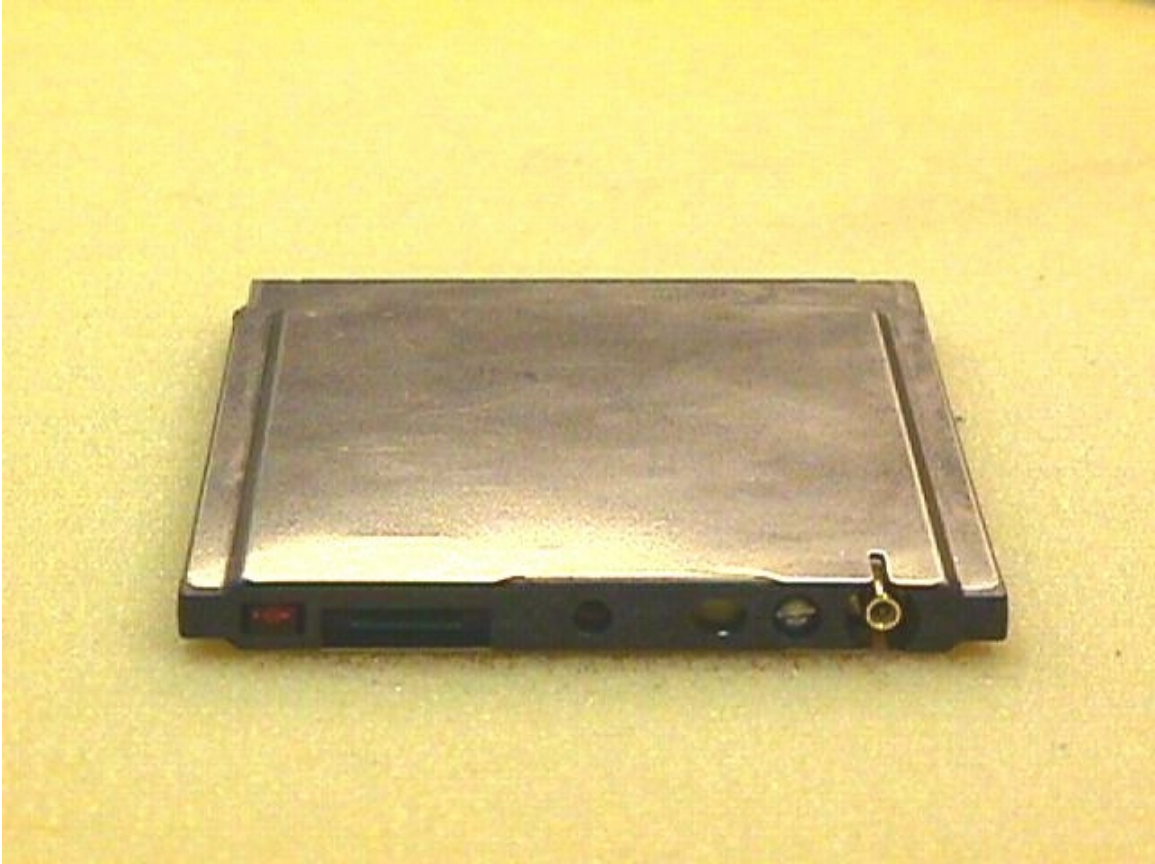
Figure 1: PCMCIA Card Edge – Outside edge showing antenna connector
