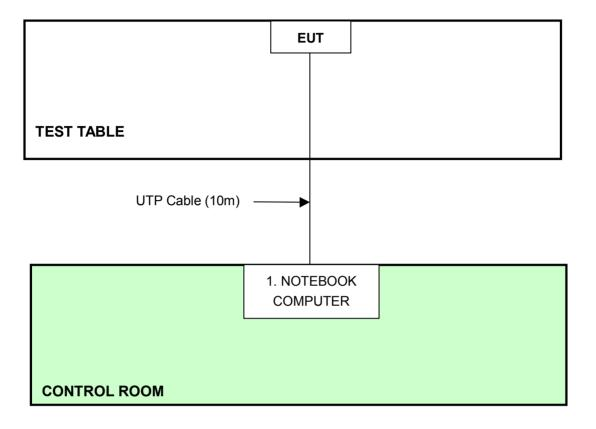
**NOTE:** 1. Support unit 1 was kept in the control room during the test.
