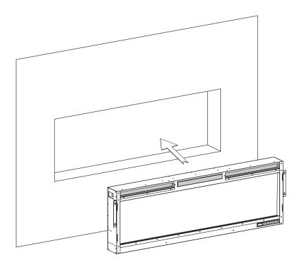
5. Attach the Firebox with 4 Large Screws (BB), on the side wood studs with an electric drill.
