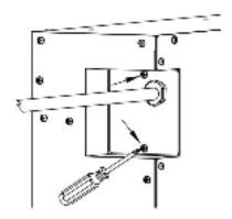
2. Pull the junction box out. loosen the screws in the terminal block to release the wires of the power cord.
