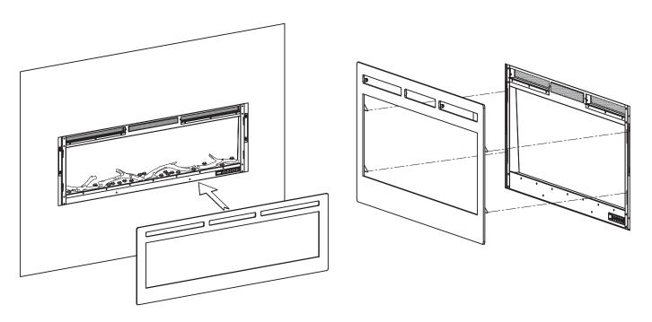
• Secure the glass front (B) by fastening 4 Small Screw (CC) and complete the installation.
