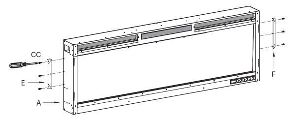
Note: The hook hole of the Mounting Bracket is on the back.
