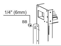
4. Lift the Firebox(A) and hang the Firebox on to the wall with the Large Screws (BB). (It's recommended that two people lift the firebox to prevent injury or damage)
