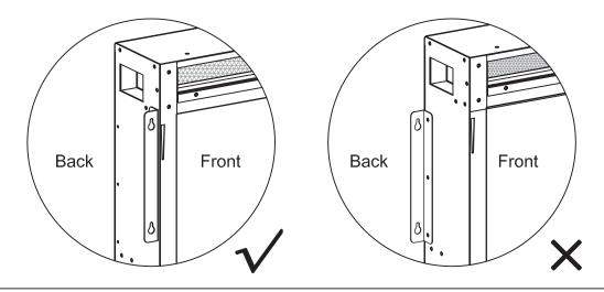
4. Insert the Firebox into the opening and adjust the position of the unit until it is centered and level.
