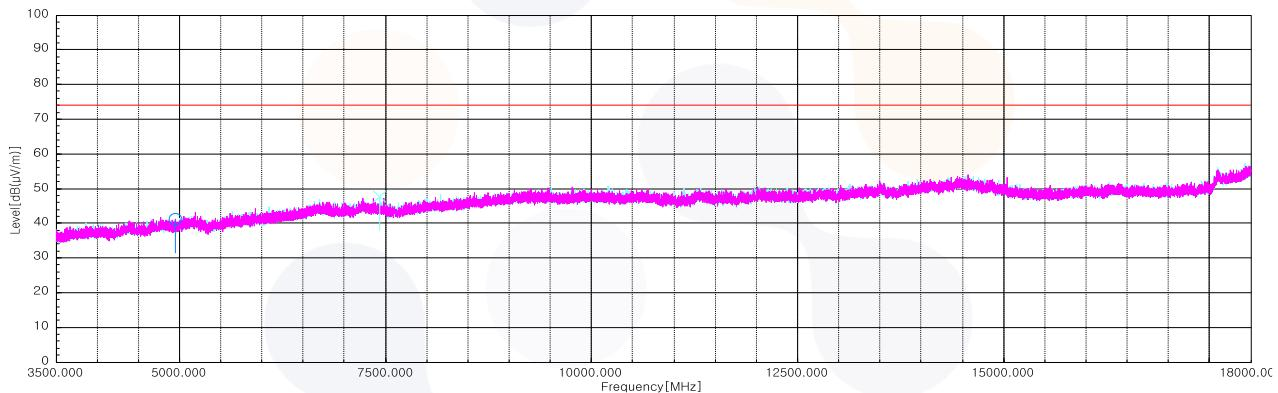
**Test results (Above 18 GHz) – Worst case: ANT1\_1 MBits/s(37 Bytes) 2 480 MHz****Horizontal/Vertical for 18 GHz ~ 26.5 GHz**
