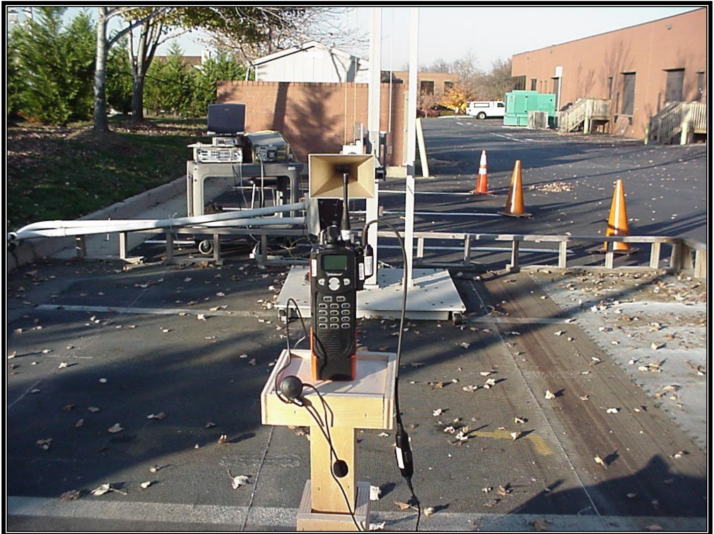
PHOTOGRAPH 3: RADIATED EMISSIONS REAR VIEW (ANTENNA MOUNTED ON RADIO)
