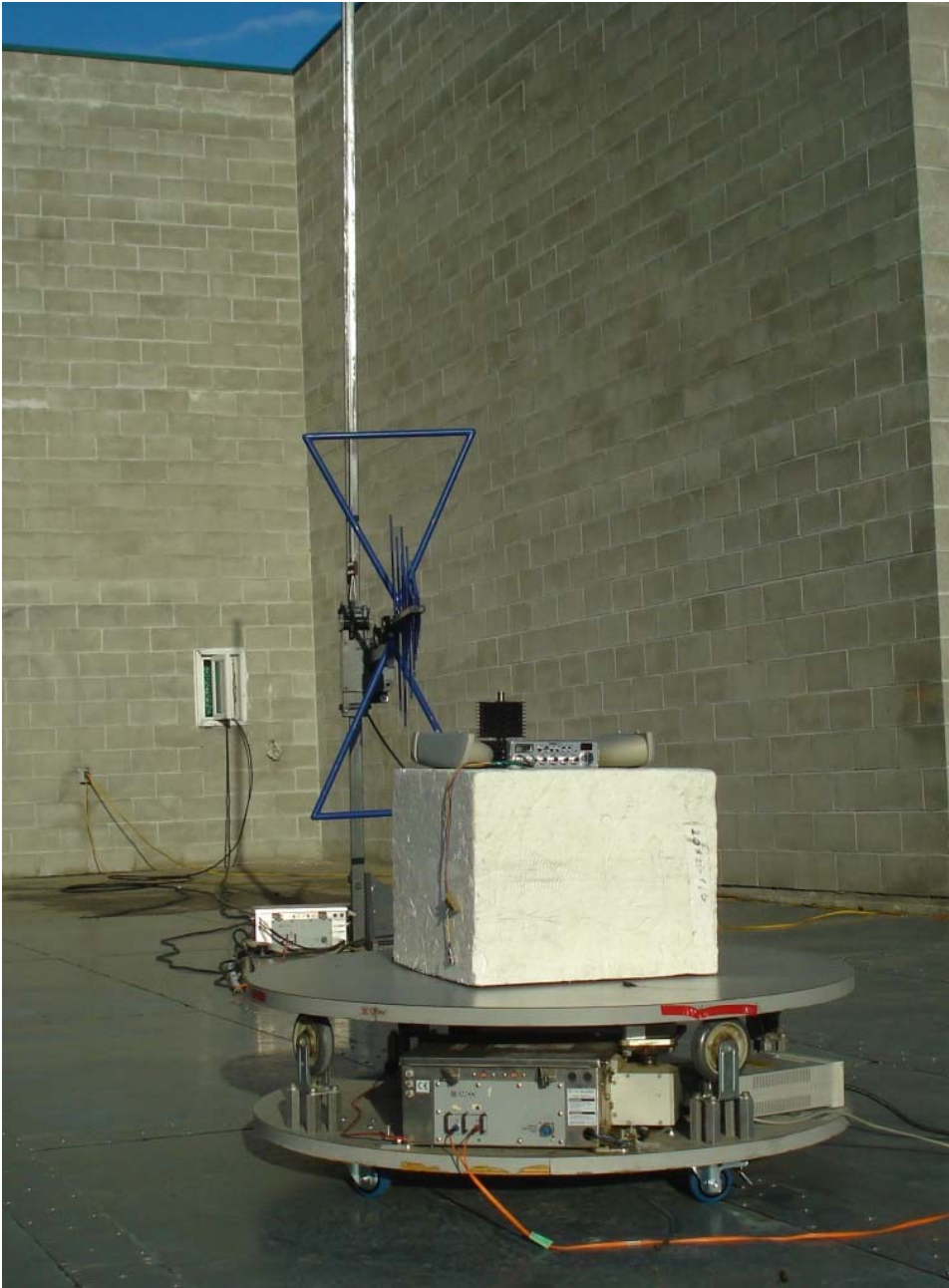
P1 – Radiated Emission on OATS
