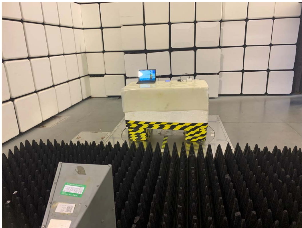
Picture 1: Radiated Emission Test Setup
