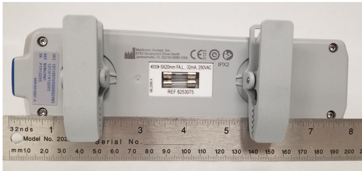
Figure 3 NIM Vital Patient Interface NIM4CPB1 Bottom View with dimensions
