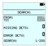
After all programmed detonators has been searched for and the test is complete, the PU displays a summary of **SEARCH MISS** test.
