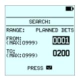
To change the range start and stop value, select the value you want to change (From or To) by pressing —/—and use the numerical buttons to enter the value.
