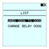
Press 🌬 and 🗖 to select the UNDO function and to display screen below which asks to confirm deleting the last 3 programmed detonators using 🗖 or to cancel with 🛤 and to return previous screen.
