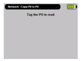
Tag the PU of which the data has to be recovered (source PU) with the DRB2.
