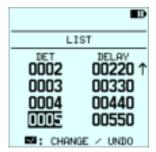
Press to exit the **LIST** function and to return to the **MAIN** operating screen to resume programming #0006.
