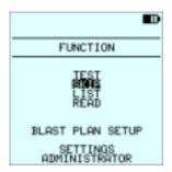
Confirm with to access screen below. Press to confirm or to cancel the **SKIP** function and to return to MAIN programming screen.
