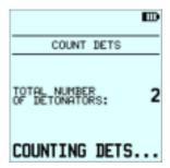
At the end of the test, the PU displays the number of detonators detected. The number of detonators detected must correspond to the number of detonators programmed. Exit to the **MAIN** operating window by pressing.
