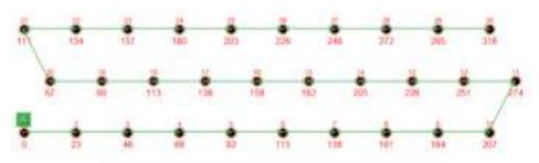
Example of a blast plan displaying sequence numbers and delays
