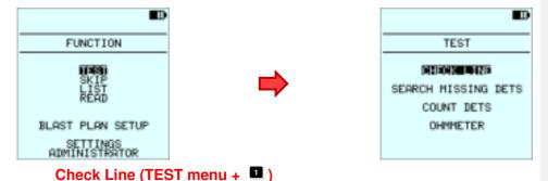
Note: The CHECK LINE function can be done with any PU and no need to use the PU used to program that section of the shot.
