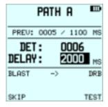
Press to access the **FUNCTION** menu and use - to select **ADD**. Confirm with to access screen below:
