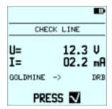
Residual current consumption of the detonators connected on line is given in the tablebelow. Always check that measured voltage is **not zero**. Maximum consumption combined with zero voltage indicates a short-circuit ( 00.0V and 20.0mA).
