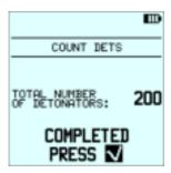
The **COUNT DETS** test can be stopped by pressing, and the function is then exited by acknowledging the interruption message by pressing.
