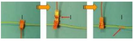
Invert the position of the connector while keeping the bus line in the same position, and reconnect a few cm further
