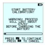
If the button is pressed or after 5 minutes, the PU proceeds automatically with standard charging.
