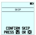
If operator has pressed the , the PU skips the current sequence number and displays the following sequence number and detonator to be programmed.
