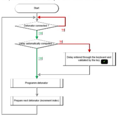
WARNING: THE DETONATORS SHOULD NOT BE REMOVED UNTIL THE PROGRAMMING IS COMPLETED BY THE PU (i.e. until you hear the 2 beeps, the PU requests the removal of the detonator or if the sequence number of the next detonator sequence number is displayed).
