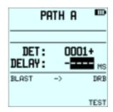
Enter the delay and connect the detonator to the PU or bus line dependant to the current connection mode.
