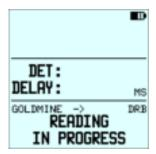
The screen below is displayed indicating the detonator's sequence # and its corresponding delay. Press to return to the **MAIN** operating screen without changing the delay, or press to change the delay. Enter the new detonator delay using the keypad and press to program it. The PU then returns to the **MAIN** operating screen.
