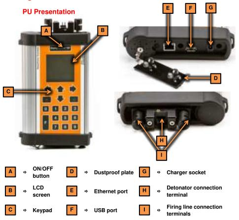
The PU has 3 connection points which are accessed by removing the dustproof plate at the bottom of the PU (simply pull on the 2 fast opening terminals): an Ethernet connection, a USB connection and a charging point.
