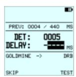
If the connected detonator has been previously programmed, the PU is capable of recognizing it and will prevent it from being programmed again. A long beep will sound and a message *PREV*. *PROGRAMMED* will prompt the operator to modify the delay if needed: press to change the delay or disconnect the detonator to avoid modifying its delay and to return to previous screen.
