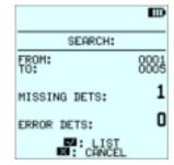
Any detonators added to the programming – usually in AUTO mode - are checked by selecting the Range option and scrolling across to select Added Dets
