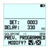
When the **READ** function is used on a detonator that has not been programmed yet by the PU, screen below is displayed showing is unique identity number. Escape the function by pressing.
