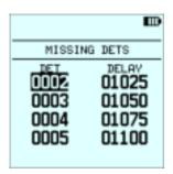
Use the **↑** and **↓** arrow buttons to scroll up and down the list or press **■** to exit.
