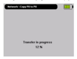
When the message "*Transfer OK*" is displayed for the second transfer, the process is completed. The blast plan has been transferred from the source PU to a target PU.
