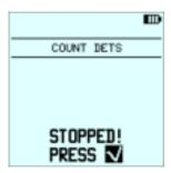
IMPORTANT: The number of detonators that can be detected by the COUNT DETS function depends on the length of the detonator wires, refer to the table above.
