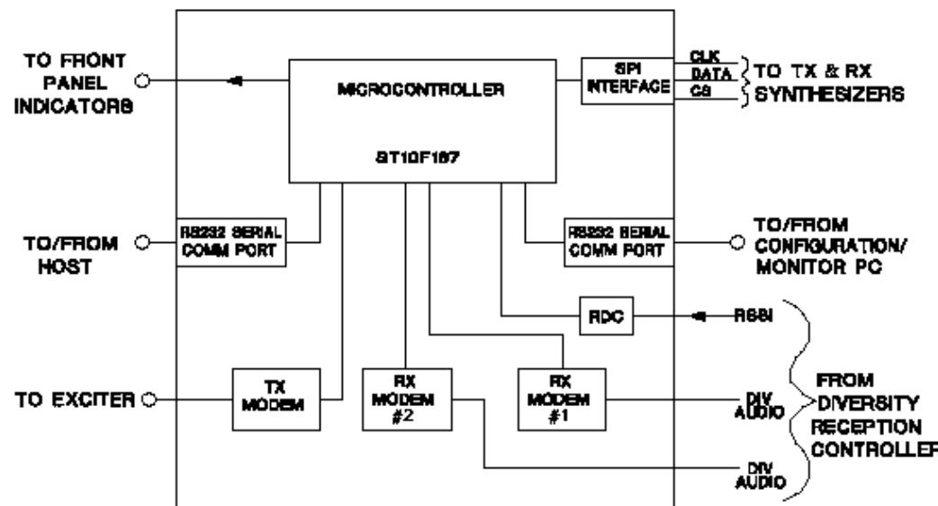
*Functional block diagram of the System Controller*
