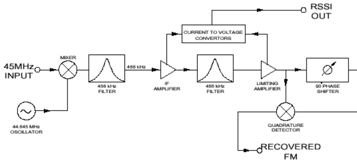
*Functional block diagram of the 45 MHz Receiver*
