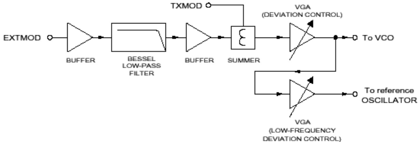
*Functional diagram of the IP1B's transmit baseband processing section*
