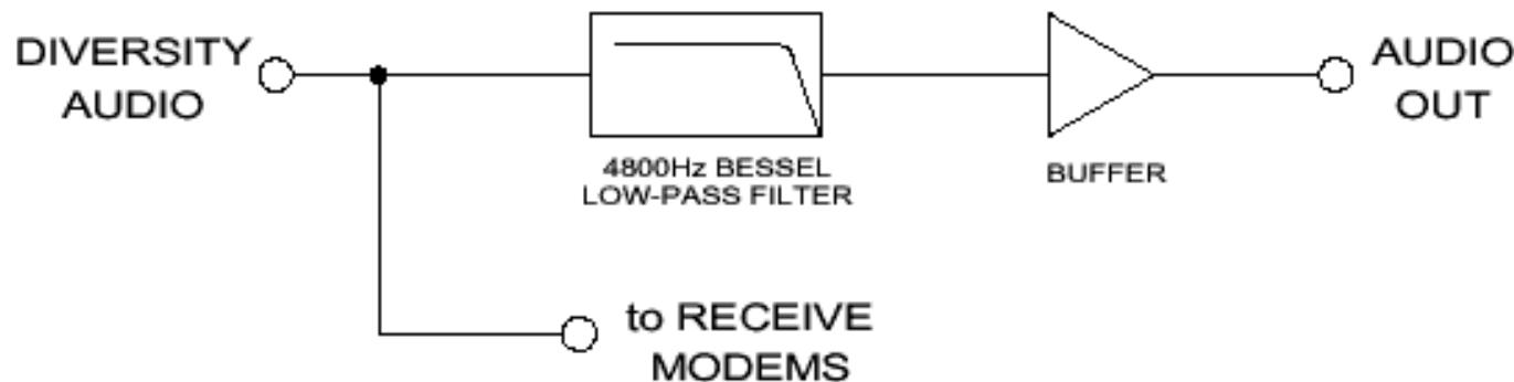
*Functional diagram of the receive baseband processing section.*
