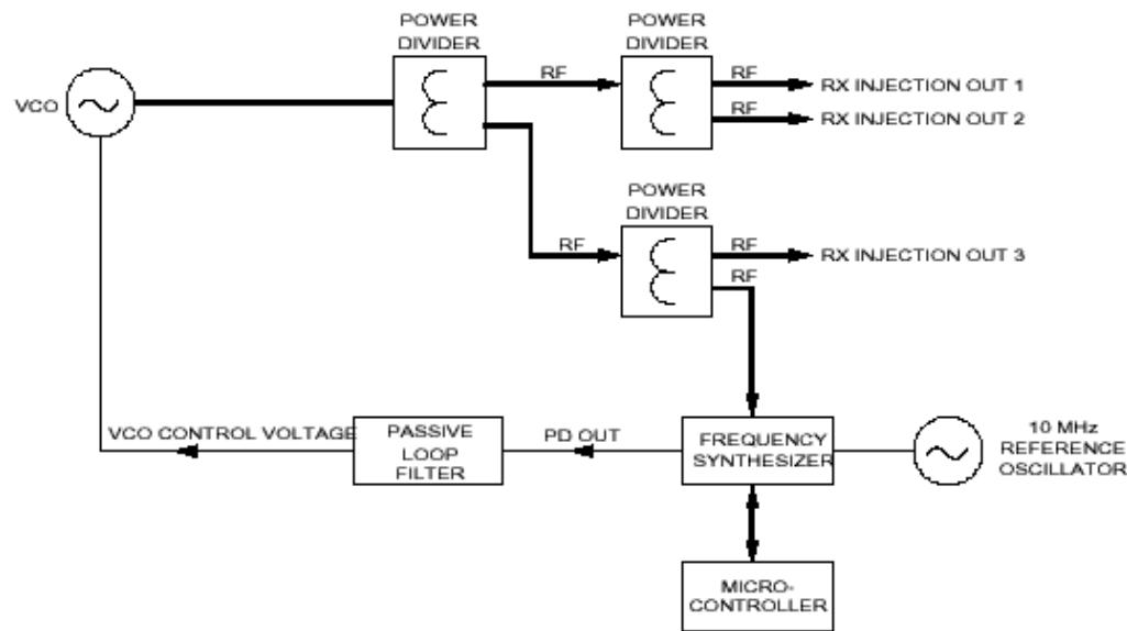
*Functional block diagram of the receiver injection*
