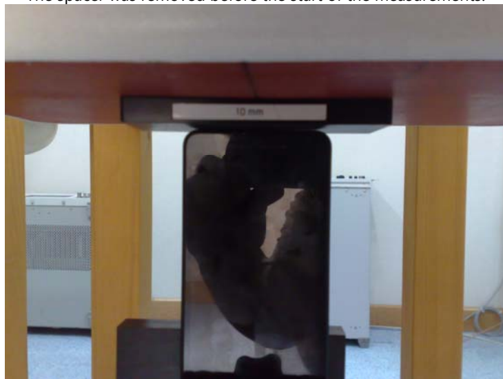
Photo of the device positioned for WR mode measurement – top edge facing phantom. The spacer was removed before the start of the measurements.
