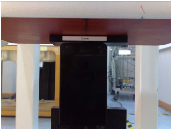
Photo of the device positioned for WR mode measurement – top edge facing phantom. The spacer was removed before the start of the measurements.
