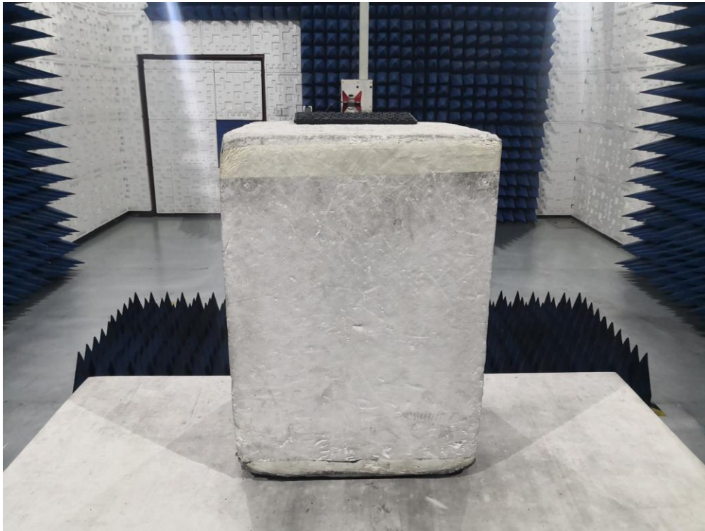
RADIATED EMISSION TEST SETUP ABOVE 1GHz
