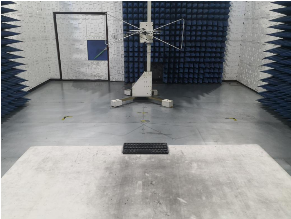
RADIATED EMISSION TEST SETUP ABOVE 1GHz
