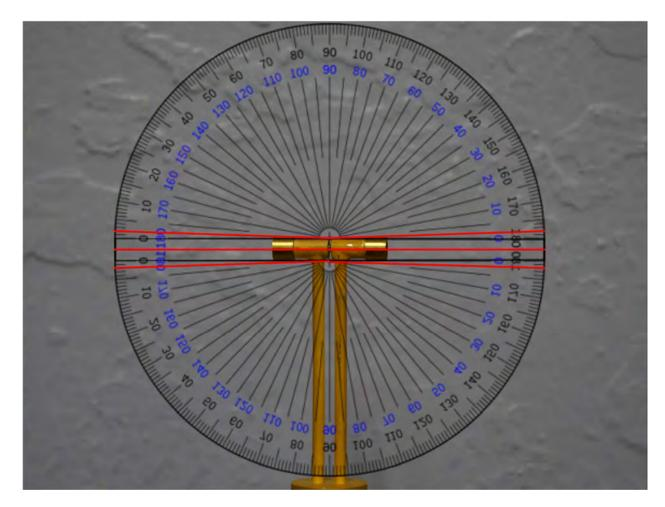
• The center red line indicates that the arms of the dipole fall within  $\pm 2^{\circ}$
