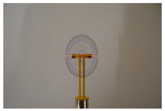
• The center red line indicates that the arms of the dipole fall within  $\pm 2^\circ$
