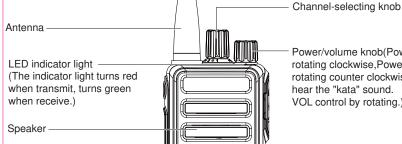
Power/volume knob(Power on by rotating clockwise, Power off by rotating counter clockwise till hear the "kata" sound. VOL control by rotating.)
