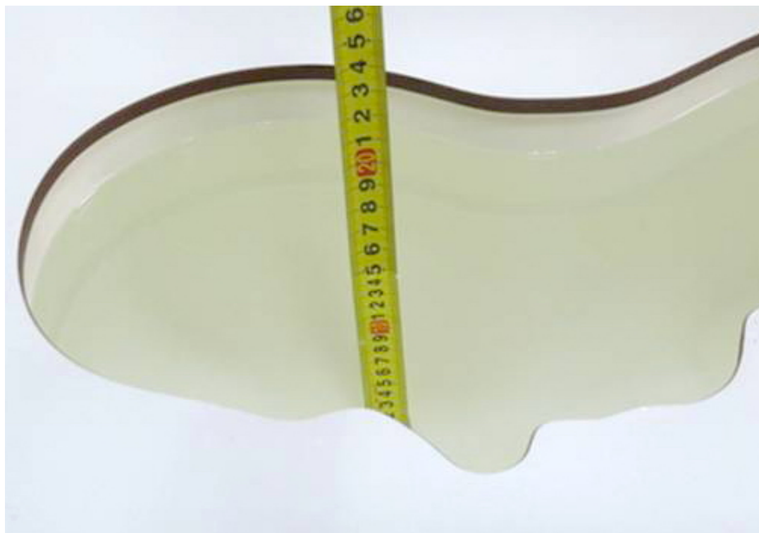
Picture 8: Liquid depth in the head Phantom (2450 MHz, 15.4cm depth)
