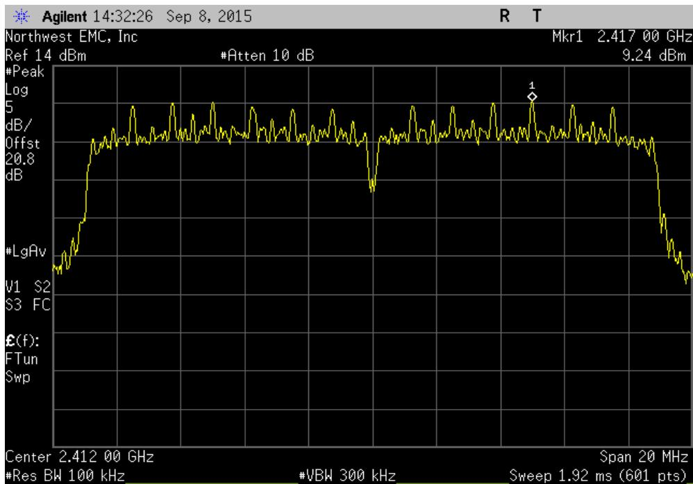
Chain B, 20 MHz, 2400 MHz - 2483.5 MHz Band, 802.11(n) MCS16, Mid Channel 6, 2437 MHz
