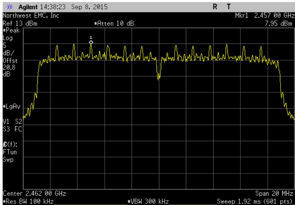
Chain B, 20 MHz, 2400 MHz - 2483.5 MHz Band, 802.11(n) MCS23, Low Channel 1, 2412 MHz
