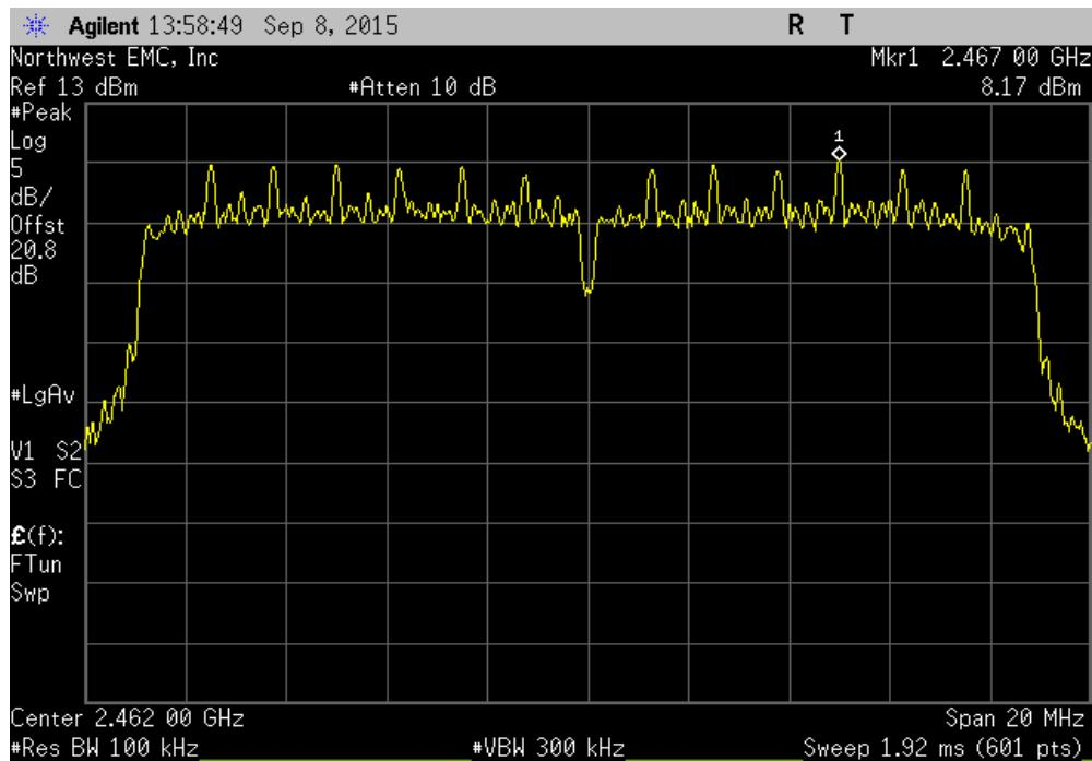
Chain C, 20 MHz, 2400 MHz - 2483.5 MHz Band, 802.11(n) MCS15, Low Channel 1, 2412 MHz
