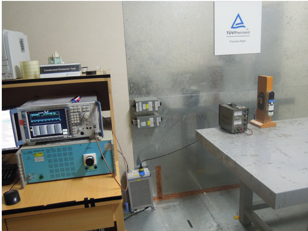
Photograph 6: Set-up for Main Emissions (Back View)
