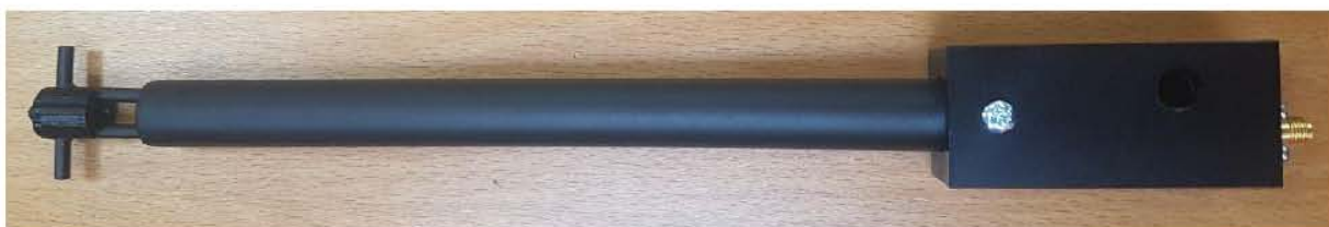
Figure 1 – MVG COMOSAR Validation Dipole
