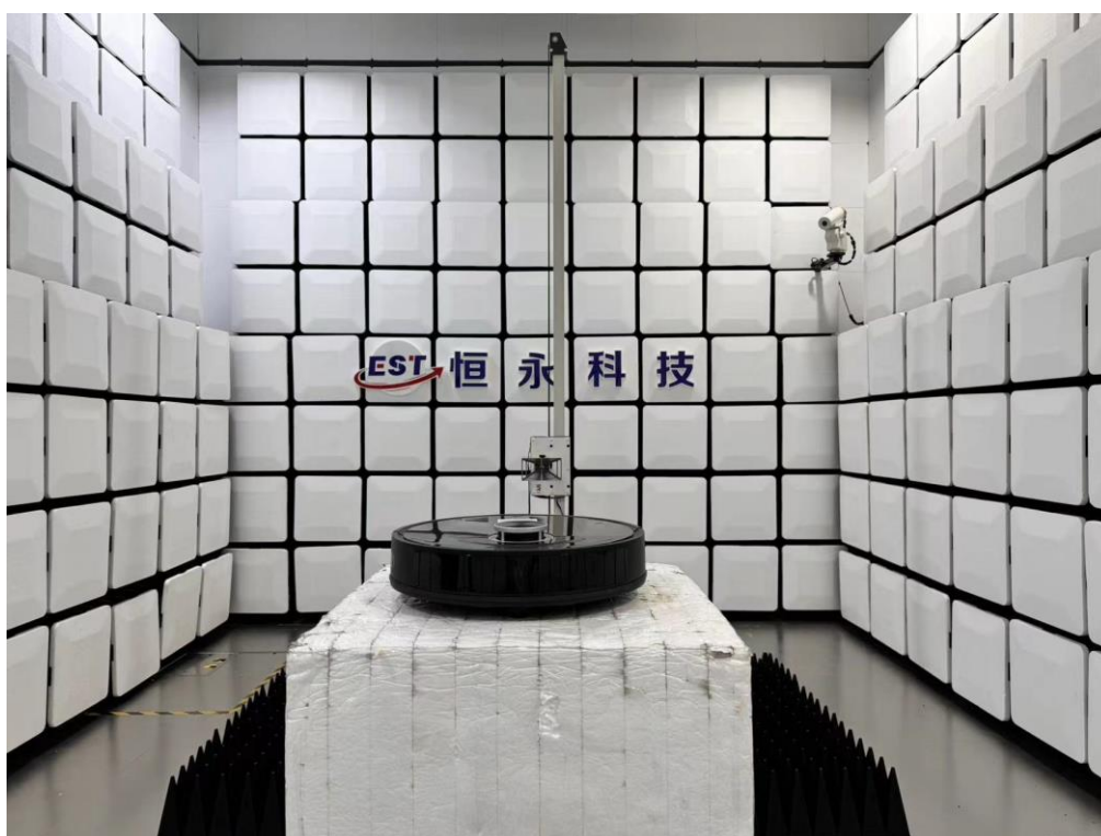
Radiated emission test: Above 1GHz
