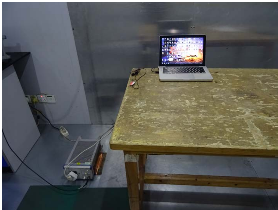
Photograph – Conducted Emission Test Setup
