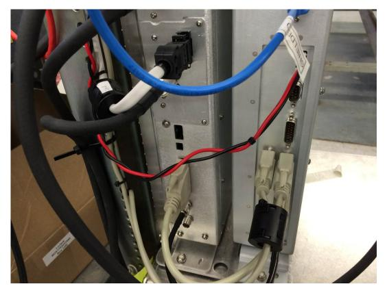
Modifications - Ferrites (Part # documented by the client) on cables as shown in photos prior to testing
