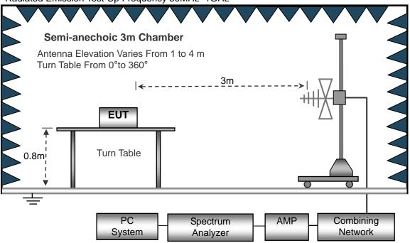
(C) Radiated Emission Test-Up Frequency Above 1GHz
